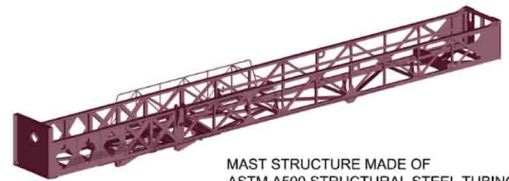
MAST STRUCTURE MADE OF ASTM A500 STRUCTURAL STEEL TUBING
